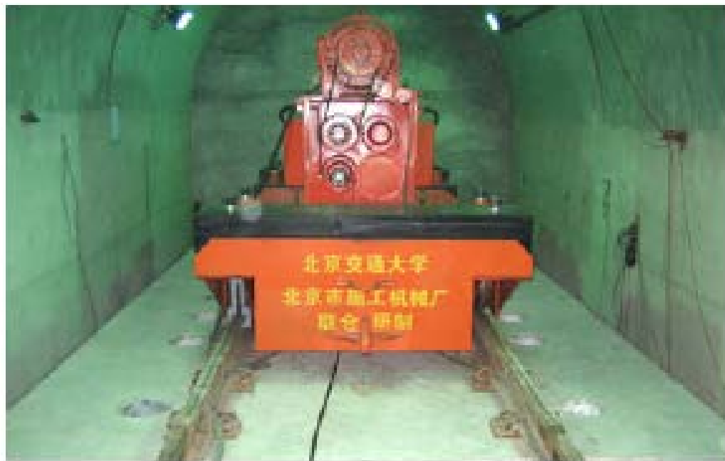
Figure 10: Unbalanced shaker used in the experiment [67].
