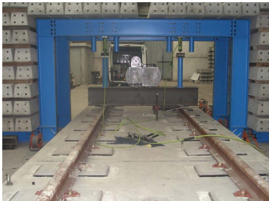
Figure 11: FST prototype used in the experimental measurement [68].
