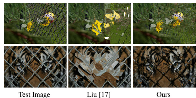
Fig. 11 Examples where Liu et al. [17] de-fencing approach fails in fence detection or in removal phase. (These test images are borrowed from Liu dataset: http://vision.cse.psu.edu/research/imageDe-fencing/index.shtml )
