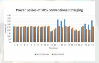
Figure 3. Power losses for 50% conventional charging
