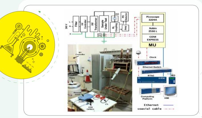
Figure 2. Experimental setup for PD detection and reporting
