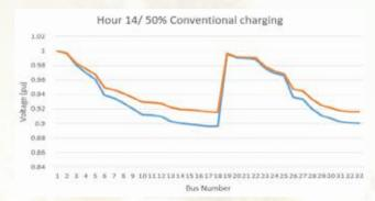
Figure 4. Voltage profile for hour 14 as conventional charging
