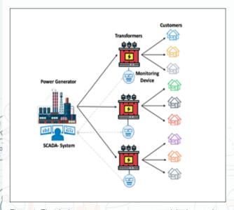
Figure 1. Electrical power system components and the invented transformer-monitoring device
