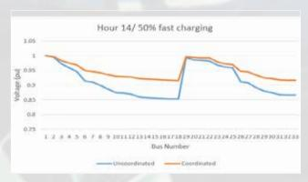
Figure 6. Voltage profile for hour 14 as fast charging
