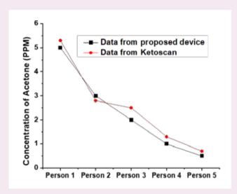
Figure 1. Comparison of data from the kit and Ketoscan demonstrating good accuracy of the kit
