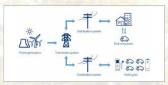
Figure 7. Vehicle to grid (V2G) and Vehicle to home (V2H)
