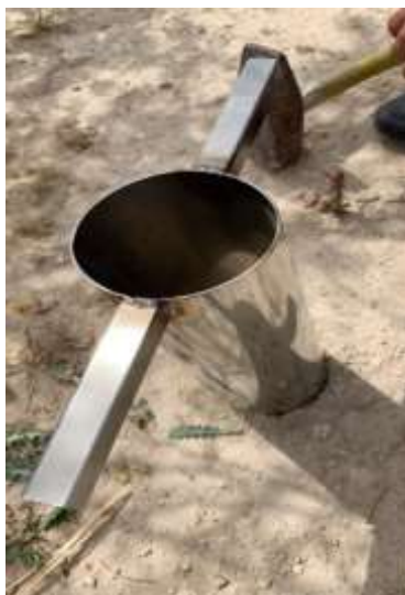
Figure A. 1 a metal core borer of 10 x 20 cm that used to collect rhizosphere sample.
