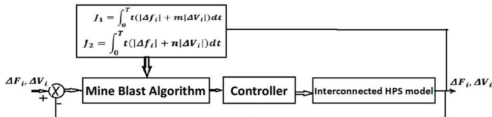
Fig. 3(d). Tuning of controllers' parameters of 3-area interconnected hybrid power system.
