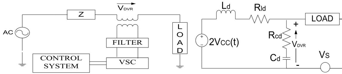
Fig. 2. Schematic with equivalent circuit structure of DVR.
