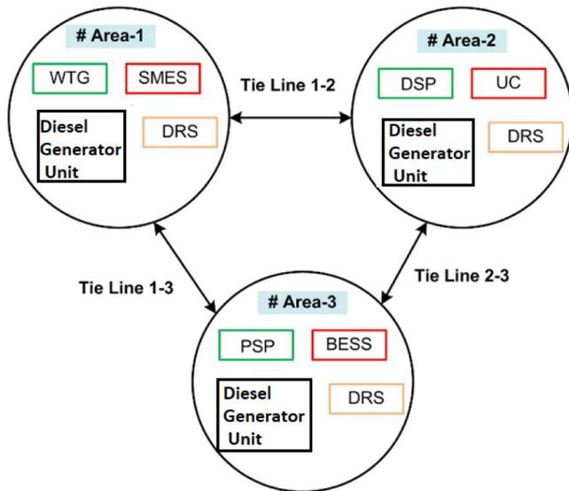
Fig. 3(a). Schematic diagram of the isolated HPS.
