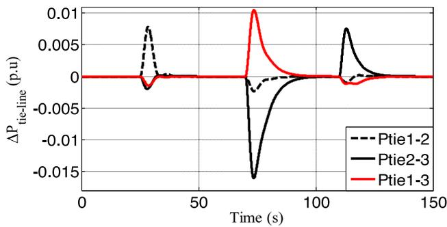
Fig. 7(c). Transient behavior of the tie-line power.
