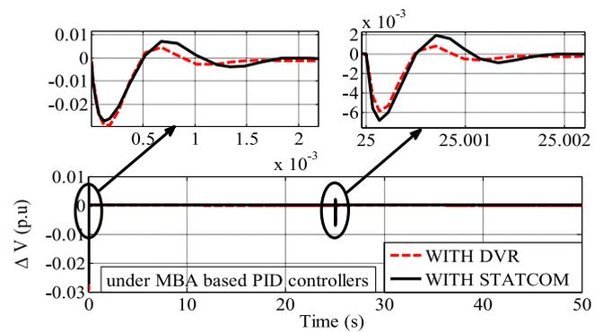
Fig. 6(b). Voltage response for direct coupling analysis.
