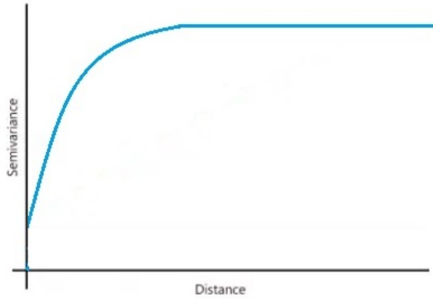
Figure 2.8: Pentaspherical variogram model
