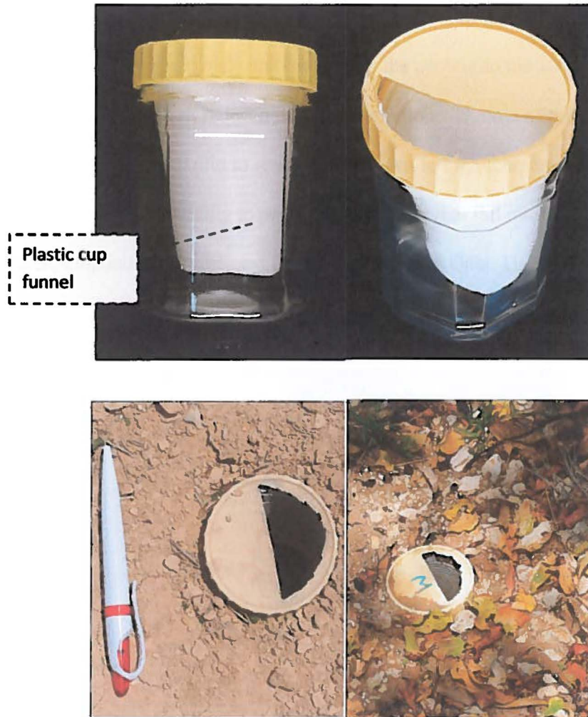
Fig. 3. Pitfall traps used in the study showing the cut lid, the cup funnel and placement in the ground.
