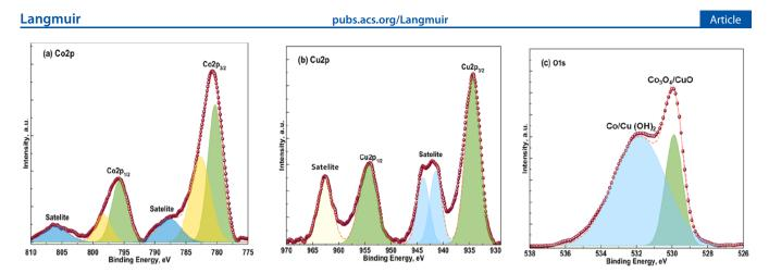
Figure 2. (a) XPS diagram showing BE levels of the  $Co_3O_4$  phase of mixed  $Co_3O_4/CuO$ . (b) BE levels of the CuO phase of mixed  $Co_3O_4/CuO$ . (c) BE of oxygen.
