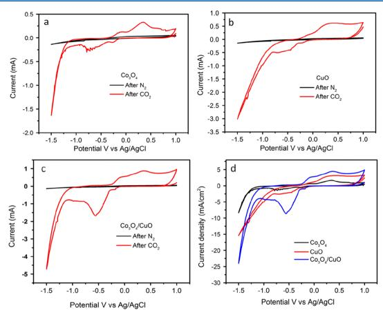
Figure 8. Cyclic voltammogram showing the study of (a)  $Co_3O_4$ , (b) CuO, and (c) mixed  $Co_3O_4/CuO$  after  $N_2$  purge and methanol (0.5 M) in 0.5 M KHCO<sub>3</sub>. (d) Cyclic voltammogram showing comparative activity of  $Co_3O_4$ , CuO, and mixed  $Co_3O_4/CuO$  of methanol (0.5 M) in 0.5 M KHCO<sub>3</sub>.
