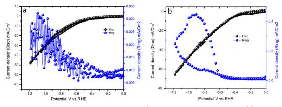
Figure 10. CV scans of  $Co_3O_4/CuO$  in 0.5 M KHCO<sub>3</sub> with the RRDE. (a) Electrolyte saturated with nitrogen and (b) electrolyte saturated with  $CO_2$ . A scan rate of 100 mV s<sup>-1</sup> and a rotation of 1500 rpm were carried out for both experiments.
