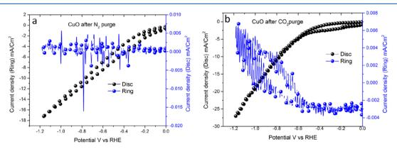
Figure 9. CV scans of CuO in 0.5 M KHCO<sub>3</sub> with the RRDE. (a) Electrolyte saturated with nitrogen and (b) electrolyte saturated with  $CO_2$ . A scan rate of 100 mV s<sup>-1</sup> and a rotation of 1500 rpm were carried out for both experiments.
