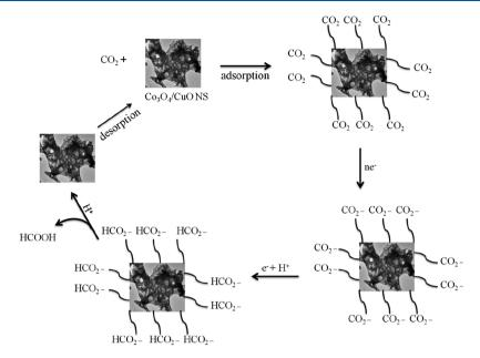
Figure 12. Transformation of  $CO_2$  to HCOOH on the  $Co_3O_4/CuO$  surface as a probable mechanism.
