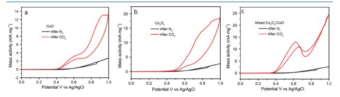
Figure 6. CV diagram showing mass activity of (a) CuO, (b)  $Co_3O_4$ , and (c) mixed  $Co_3O_4/CuO$  after  $N_2$  purge (the black curve) and 0.5 M methanol (the red curve).
