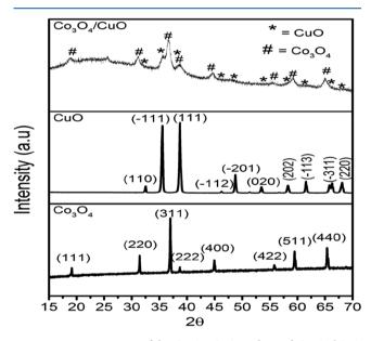
Figure 1. PXRD patterns of the Co<sub>3</sub>O<sub>4</sub>, CuO, and mixed Co<sub>3</sub>O<sub>4</sub>/CuO electrocatalysts. The  $2\theta$  values from 10 to  $80^{\circ}$  with a scan rate of  $2^{\circ}$  per min were considered during PXRD measurement.
