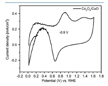
Figure 11. Ring electrode CV scan of  $Co_3O_4/CuO$ . A scan rate of 1500 rpm was taken.
