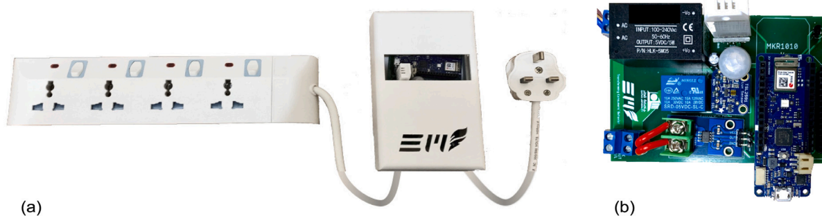
Fig. 6. Anatomy and PCB of the implemented smart plug.
