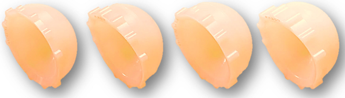
Figure 4. Different acetabular liner model designs with moderately cross-linked UHMWPE [61].
