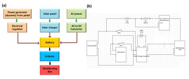
Fig. 6. (a) Flowchart of disinfection unit working based on power supply, human and solar power. (b) The circuit involved in powering the disinfecting unit.
