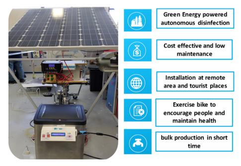
**Fig. 7.** Photograph of the developed disinfecting unit powered with green energy sources and key advantages. (For interpretation of the references to colour in this figure legend, the reader is referred to the web version of this article.)
