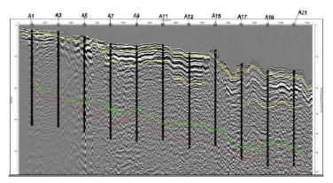
Fig. 6: Seismic reflection cross section and boreholes
