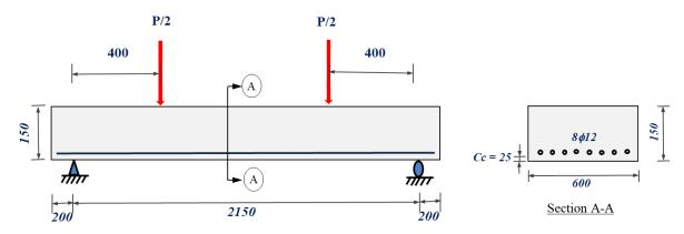
Fig. 2: Testing Set-Up. All Dimensions are in Mm
