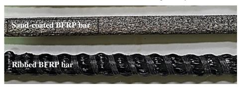
Fig. 1: The Used BFRP Bars
