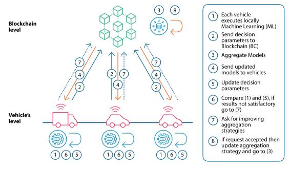
**FIGURE 3** In the proposed framework steps 1–8 on the right side of the figure describe the list of tasks from executing ML locally, followed by the aggregation and the improvement process, and finally, the sharing of final results
