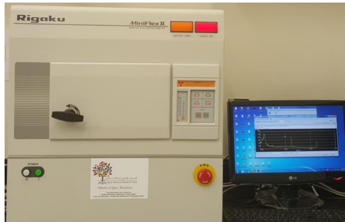
Figure 3.4: XRD instrument model: Rigaku MiniFlex II
