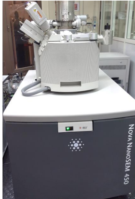
Figure 3.2: SEM instrument model: FEI NOVA NANOSEM 450
