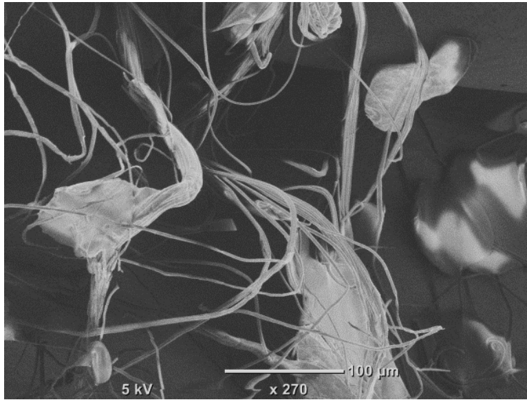
Figure 3.10: Coagulation of sulfur particles on polymer fibers
