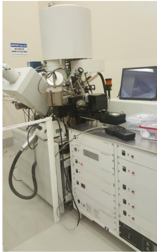
Figure 3.5: X-ray photoelectron spectroscopy model: Kratos AXIS Ultra DLD
