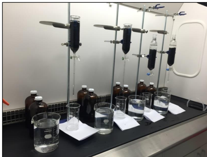
Figure 13: Activated carbon filtration columns.
