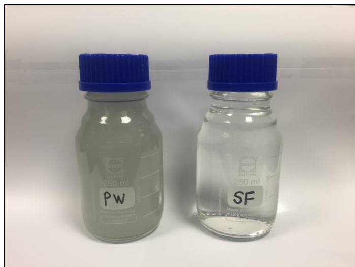
Figure 15: Produced water (PW) before and after sand filtration (SF).
