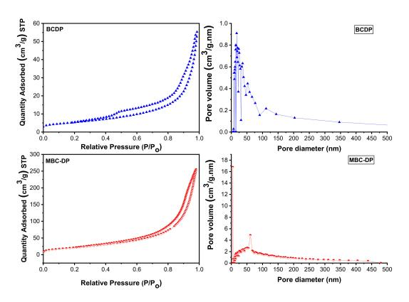
Figure 6. BET analysis of the as-prepared samples of BCDP and MBC-DP.
