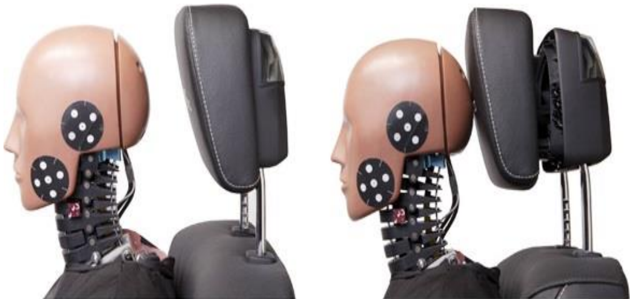
Figure 9. Example of Pro-AHR with a stationary part and moving cushion [10].
