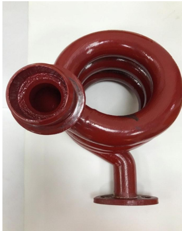
Figure 40. Induction manifold with tribled inlet diameter and 30 degress outlet angle
