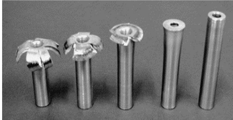
Figure 2-4: Steel circular tubes under the following velocity from right to left: 385 m/s, 277 m/s, 227 m/s, 173 m/s and 0 m/s [49]
