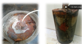
Figure 3: Crack pattern at lapped spliced joint in cylinder samples in: a) c/d = 2.6; b) c/d = 1.5.
