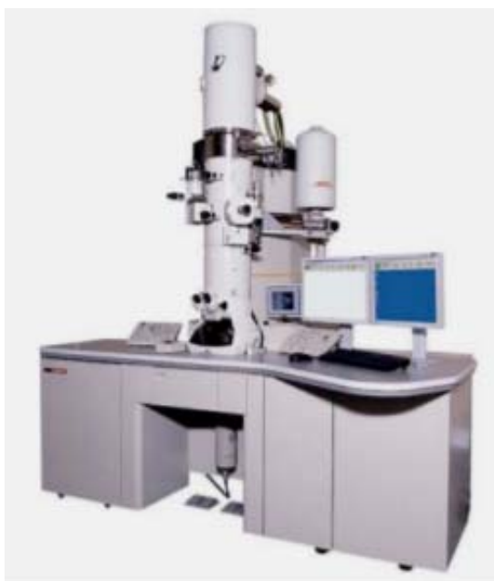
Figure 21. HRTEM device used for morphological imaging
