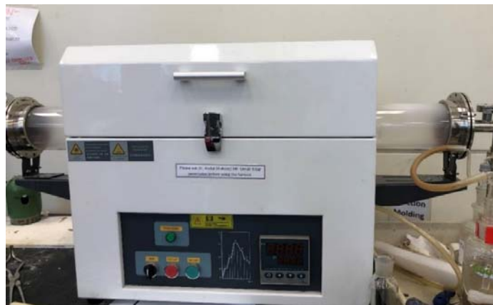
Figure 17. MTI Tube furnace used for heat treatment of deposited specimens.
