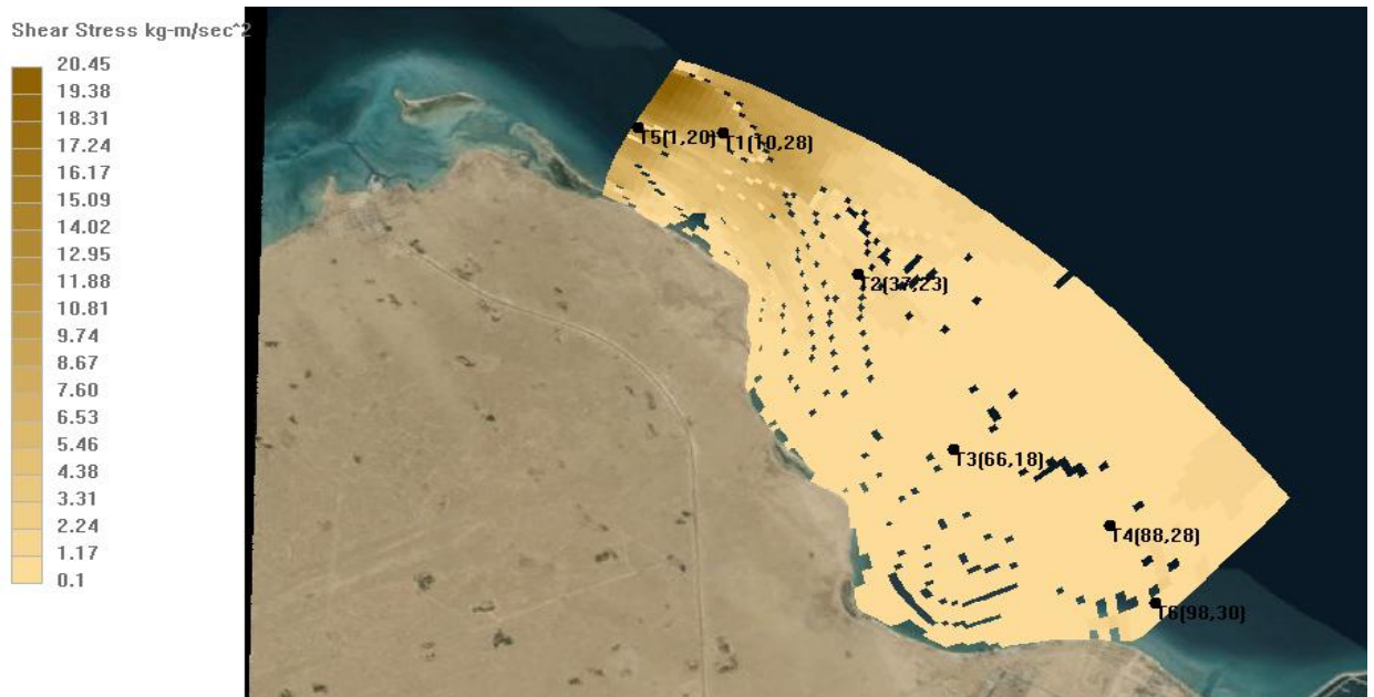
Figure 47: Scenario (1) conditions simulation for Shear stress ( \text{kg.m/sec}^2 ) in 08/1/2014 at 11:00 a.m.
