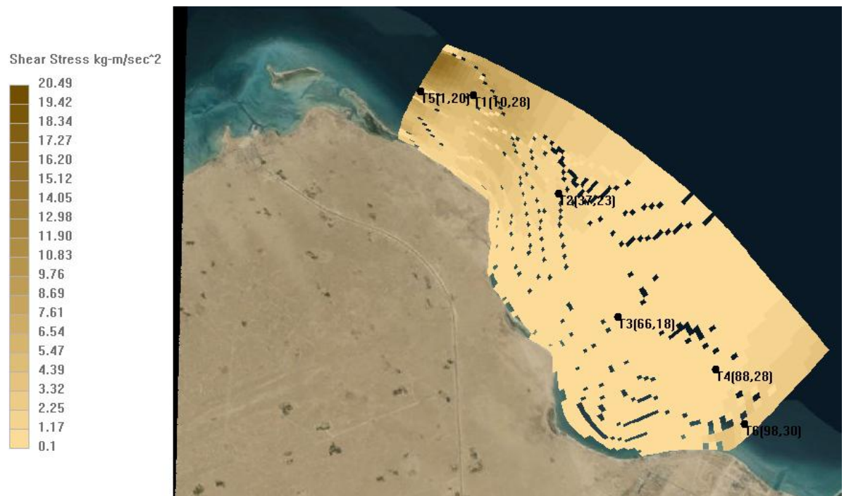
Figure 43: Present conditions simulation for Shear stress (kg.m/sec 2 ) in 08/1/2014 at 11:00 a.m.
