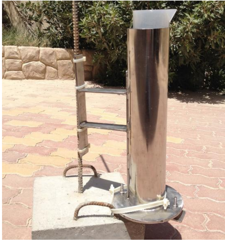
Figure 27: Sediment traps attached to concrete base to guarantee a vertical position when deployed on site
