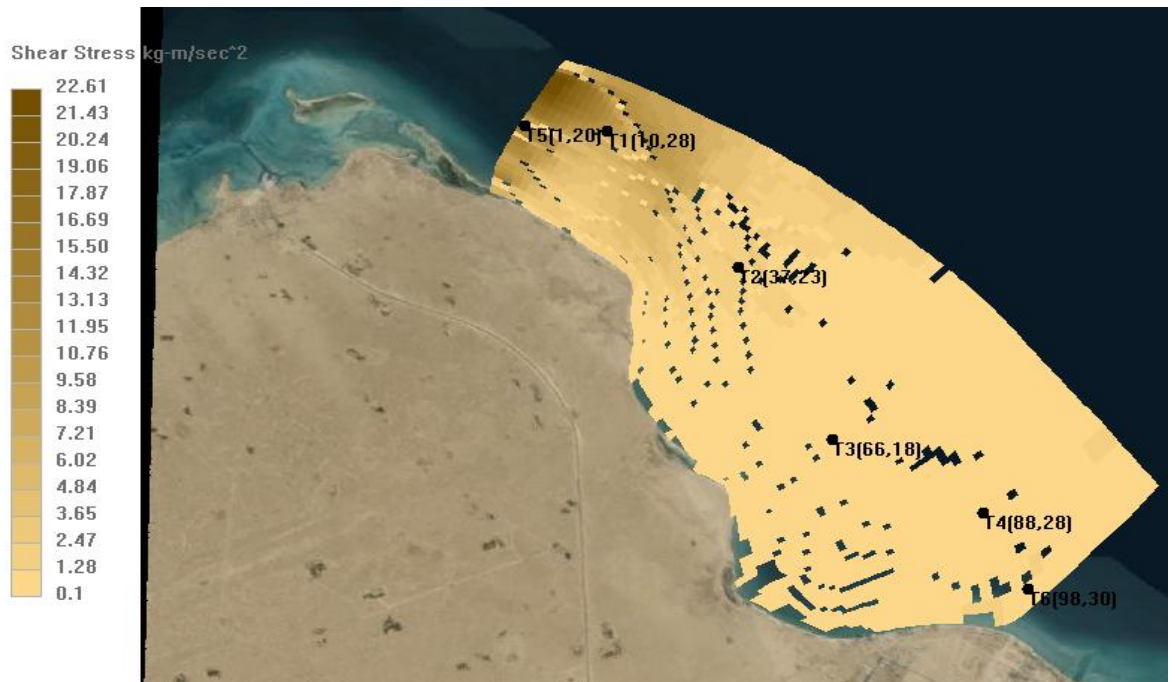
Figure 49: Scenario (3) conditions simulation for Shear stress( \text{kg}\cdot\text{m}/\text{sec}^2 ) in 08/1/2014 at 11:00 a.m.
