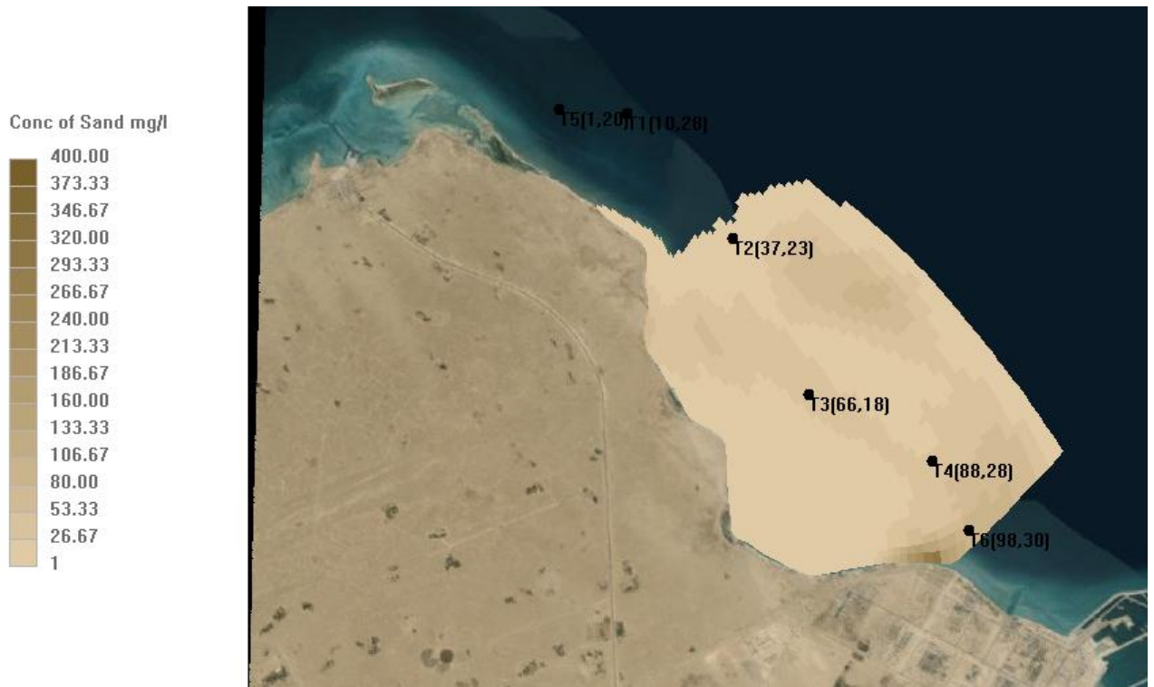
Figure 44: Present conditions simulation for concentration of sand (mg/l) 08/1/2014 at 11:00 a.m.
