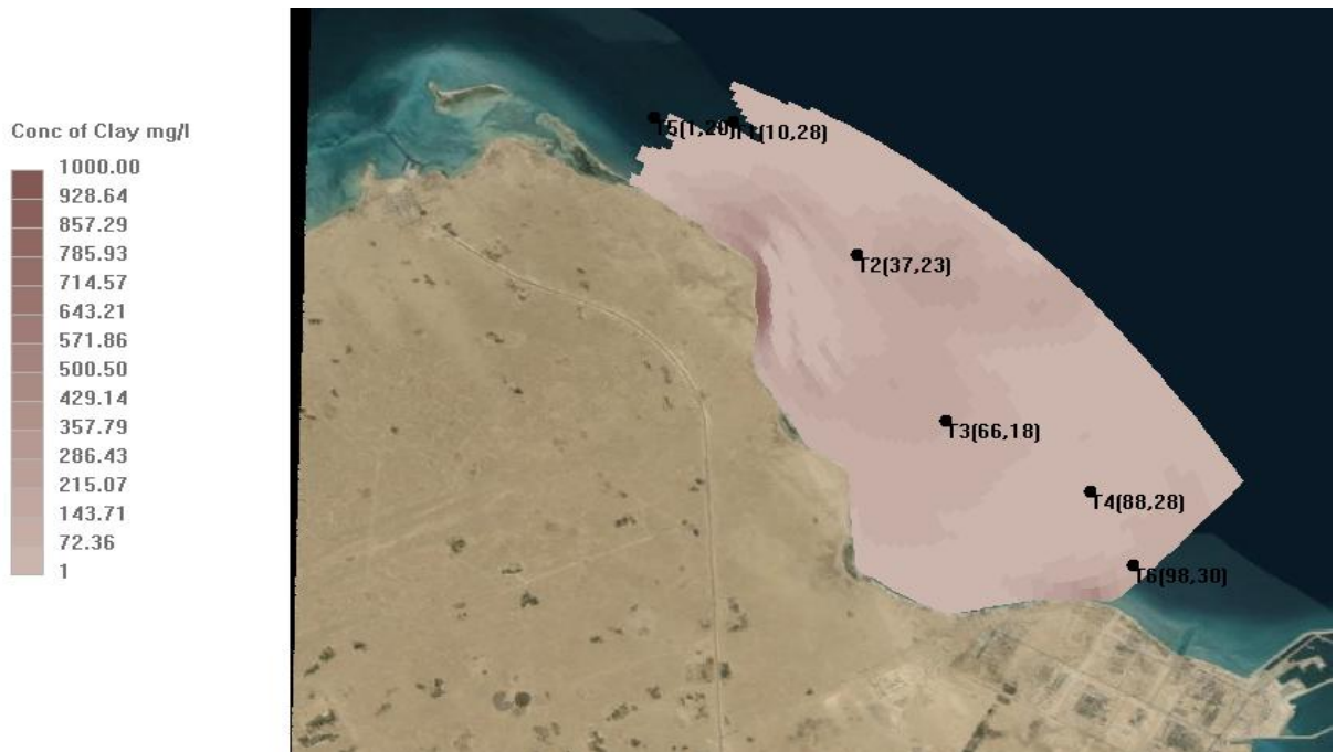
Figure 46: Present conditions simulation for concentration of Clay 08/1/2014 at 11:00 a.m.
