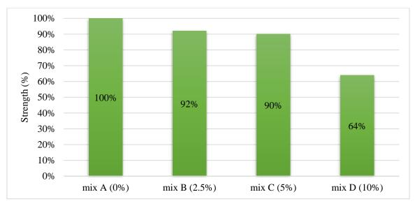
Fig. 5: Strength of Different Prisms in Comparison to the Cracking Load of the Reference Mix
