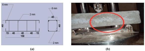
Fig. 4: Pre-cracking of Mortar Prism
