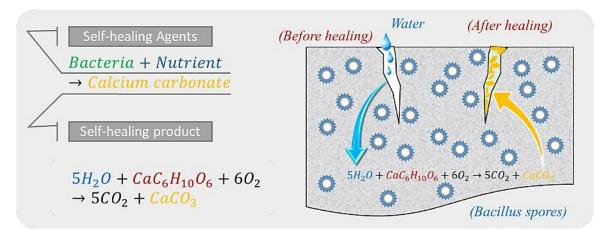
Fig. 1: Mechanism of Self-Healing Concrete
