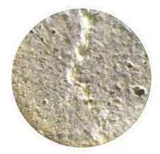
Fig. 7: 25x Stereomicroscope Image Showing the Formation of Calcite on a Crack
