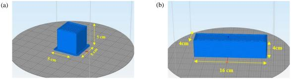
Fig. 1: (a) Details of ready-to-print 3D models of a) cube for compressive strength and b) prism for flexural strength
