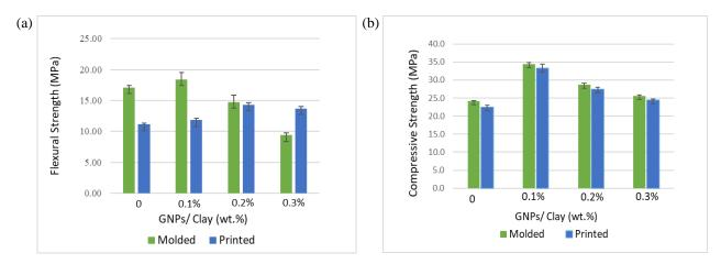
Fig. 3: (a) Flexural strength test results, and (b) Compressive strength test results
