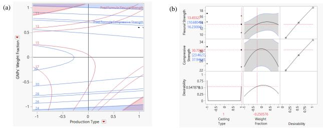
Fig. 5: (a) Production type and GNPs' weight fraction variables contour profiles and (b) maximized desirability functions
