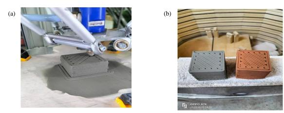
Fig. 2: (a) 3D-printing process, and (b) burnt vs unburnt sample
