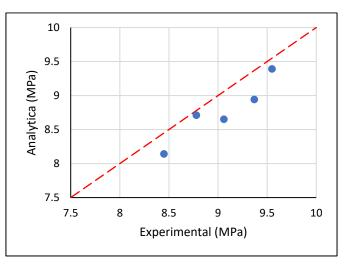
Fig. 4: Analytical vs Experimental Composite Tensile Strength of HyFR-HSC & HyGrFR-HSC
