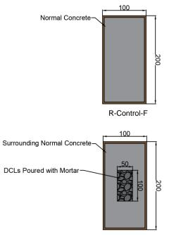
R-100x50-D19 and R-100x50-D25 Fig. 1: Section details of CFST beam specimens, dimensions in mm
