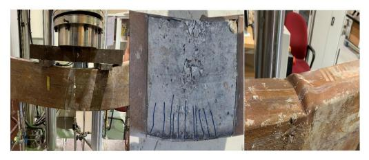
Fig. 6: Failure mode of steel and concrete
