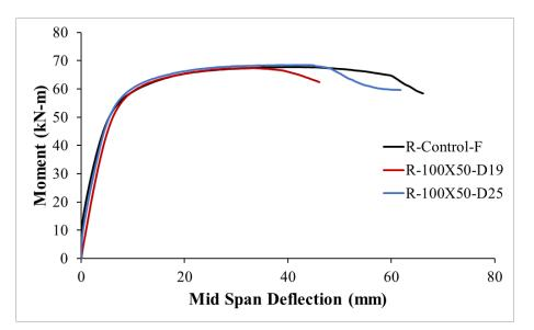
Fig. 3: Moment versus midspan deflection curves
