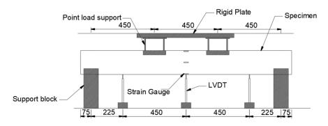
Fig. 2: Schematic test setup, dimensions in mm
