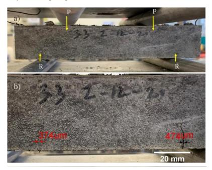
Fig. 2: a) prism samples under four-point loading for cracks formation. Crack generation in prism samples.b) Cracks up to 474 μm in the samples with *bacillus cereus*
