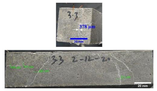
Fig. 4: The prism samples showing the self-healing of the cracks with local bacterial strains. The cracks of up to 680 microns were filled with calcium carbonates
