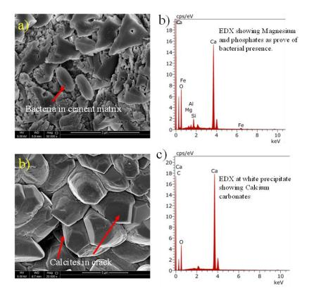
Fig. 5: a) SEM of bacterial survival in a cement matrix, b) EDX of bacterial surroundings, c) Calcium carbonate mineral (crystalline shape), d) EDX of calcium carbonate mineral
