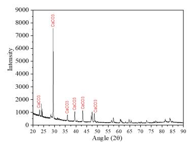
Fig. 6: XRD spectra of crack filling material in samples with local strains of bacillus cereus
