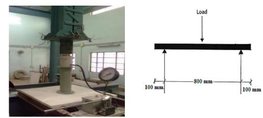
Fig. 2: Loading set up for the experimental work
