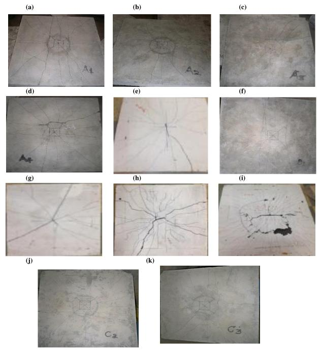
Fig.4: Cracked pattern and punching shear envelope for different slab
