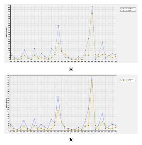
Fig. 5: Headflow at WDD downstream for (a) the WDD and (b) the WD two dams' system
