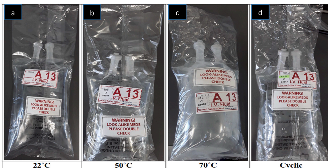
Fig. 2. Bulging effect of constant temperature at a) 22, b) 50, c) 70 °C and d) cyclic temperature on the polyolefin (PLÜMAT) packaging bags of normal saline.
