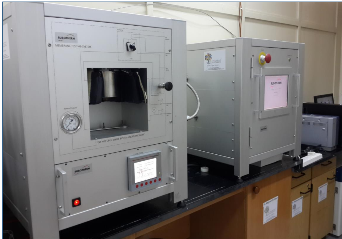
Figure C.1: Actual picture of the Rubotherm Membrane Reactor TM (System 2).
