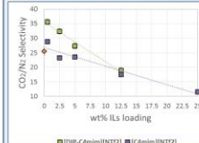
Fig 1: CO 2 /N 2 Selectivity behavior with different loads of [DIP-C 4 mim][NTf 2 ] and [C 4 mim][NTf 2 ]
