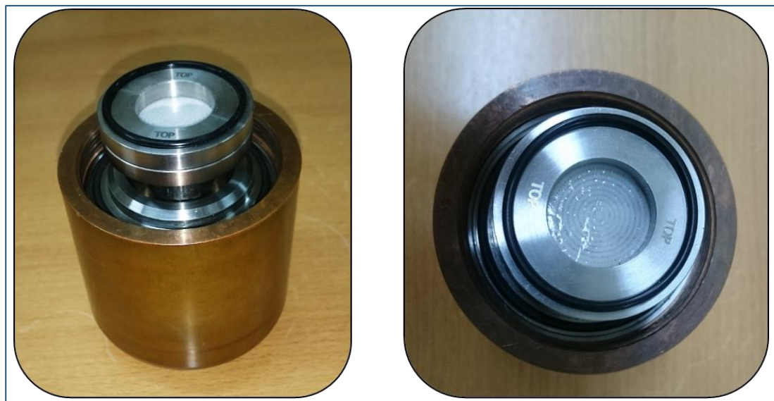
Figure C.2: Membrane holder of Rubotherm Membrane Reactor TM (System 2).
