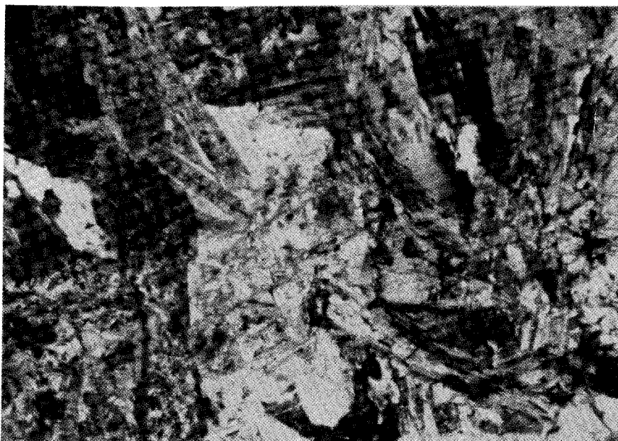
Fig. 4 Biotite granite showing deformed quartz and small crystals of kinked plagioclase enclosed in deformed alkali feldspar.
