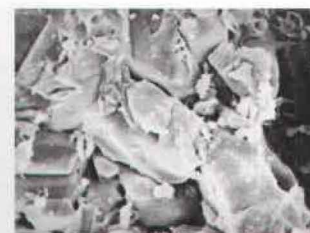
Fig. 8: Scanning electron microphotograph showing alite (grey), free lime and calcite (white). Sulphur resistant clinker, Al Ain. 1000 X
