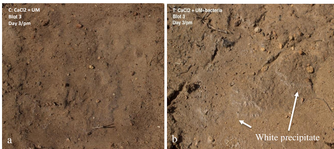
Figure 17. (a) Control; Urea Medium + CaCl 2 (b) Treatment; Urea Medium + CaCl 2 + AA2; White precipitates observed on the surface soil in blot with urea medium, calcium chloride and AA2
