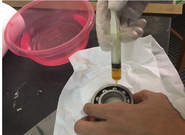
Figure 34: Applying lubricating oil to bearing after cleaning
