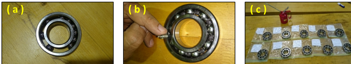
Figure 28: Remounting the bearings: (a) Replacing the balls inside the inner and outer rings, (b) Closing the bearing with rivets, (c) Lubricating the defective bearings
