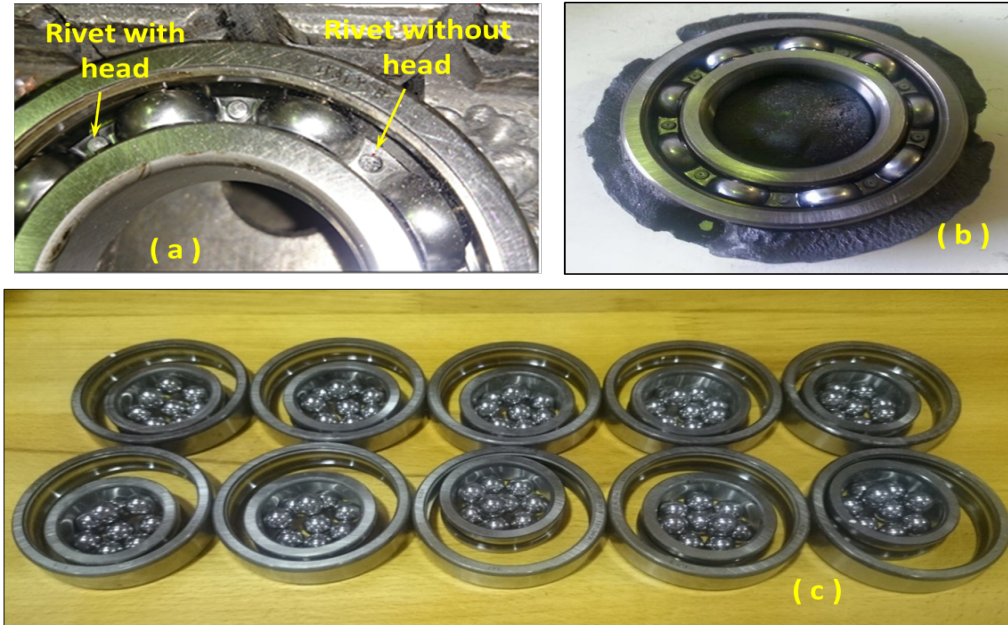
Figure 24: Dismounting the bearing: (a) Rivet head removal, (b) Epoxy clay mold to hold bearing cage, (c) Fully dismantled bearings
