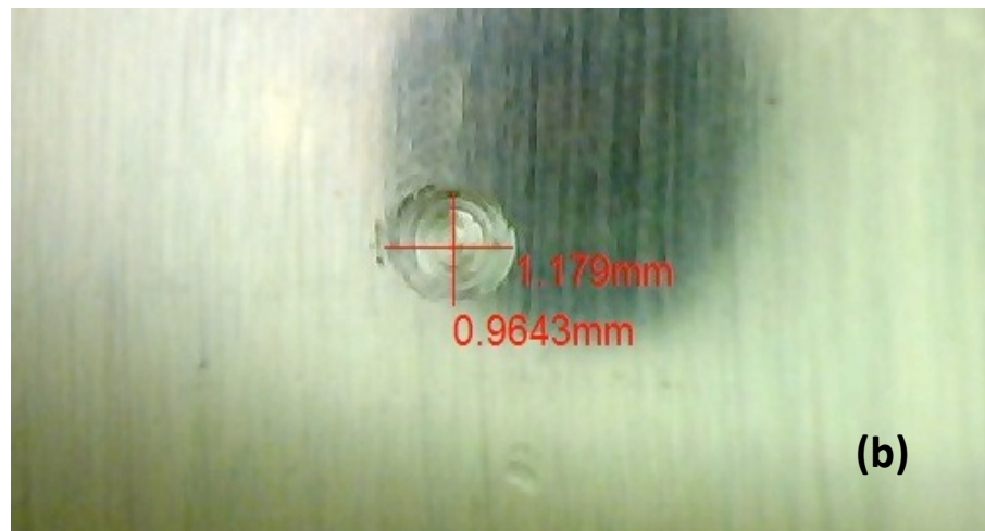
Figure 27: Microscopic observation of defects: (a) Observation of outer ring defect, (b) Shape of inner ring defect under microscope
