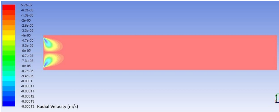
Figure 52: Radial Velocity contour of flow in Circular Tube.
