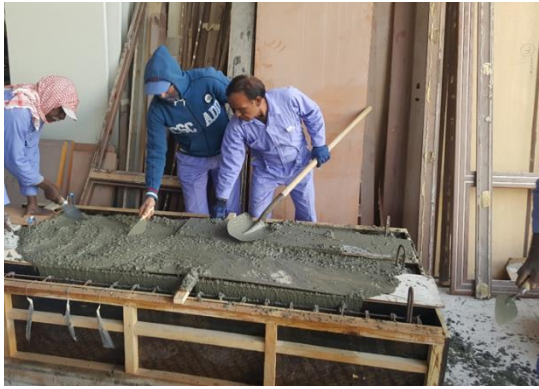
(a) Concrete casting for beam specimens
