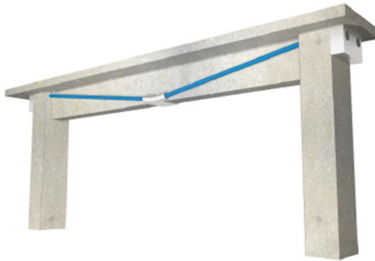
Figure 3: External post-tensioning of beam [43].
