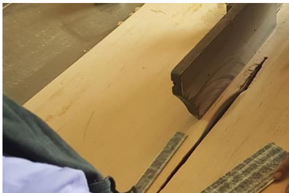
Figure 26: FRP strips cutting.
