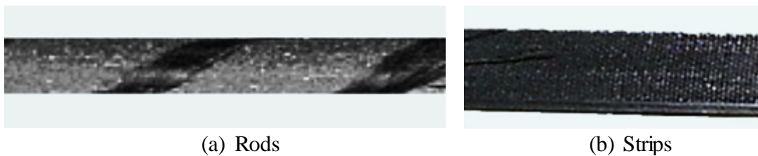
Figure 6: CFRP rods and strips [17].
