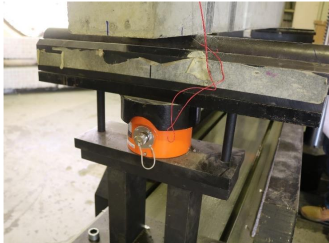
Figure 33: Load cell fixed under the support to monitor the reactions.
