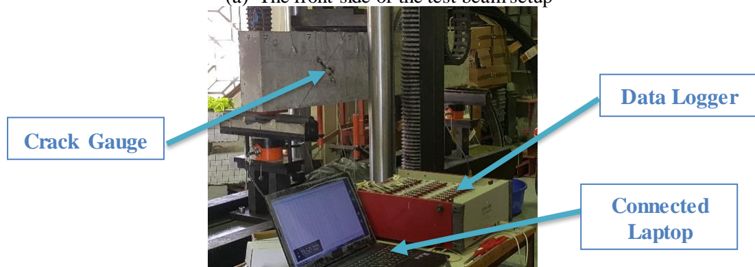
(b) The back side of the test beam setup
