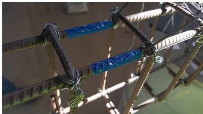
(b) Cover the strain gauges by electrical tape for protection
