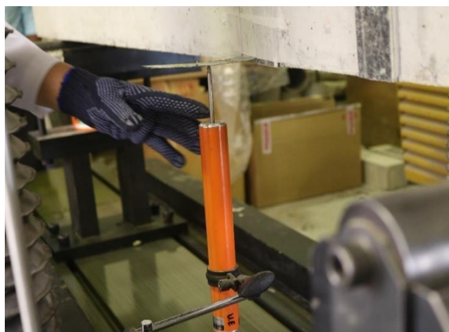
Figure 34: Linear variable displacement transducer (LVDT).
