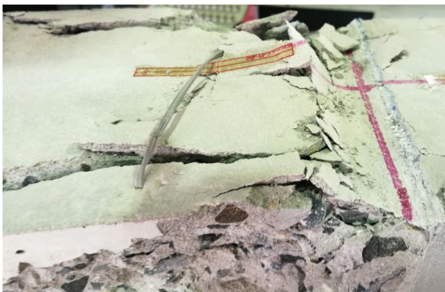
Figure 51: Concrete crushing under the loading point for specimens N3-S-C2/C1
