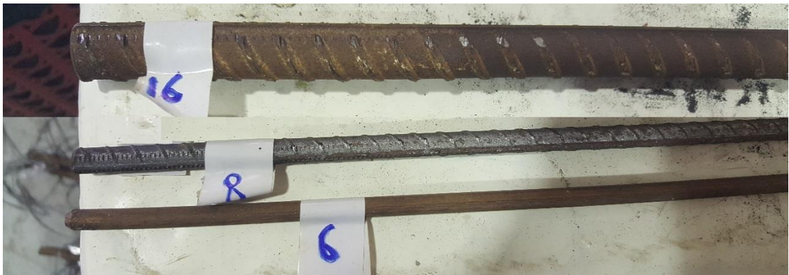
Figure 13: Steel bars used in the test; namely, 16 mm, 8 mm, and 6 mm diameter bars.
