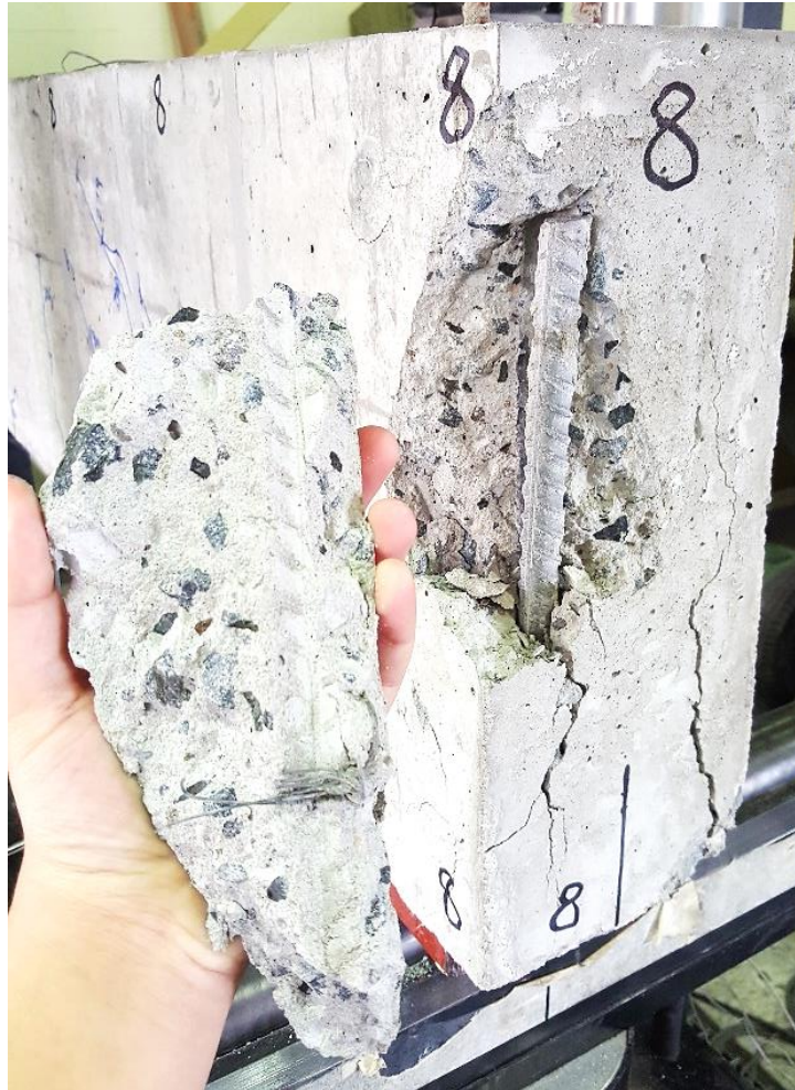
Figure 50: Broken concrete mass while testing the specimen N2-S2-C2.
