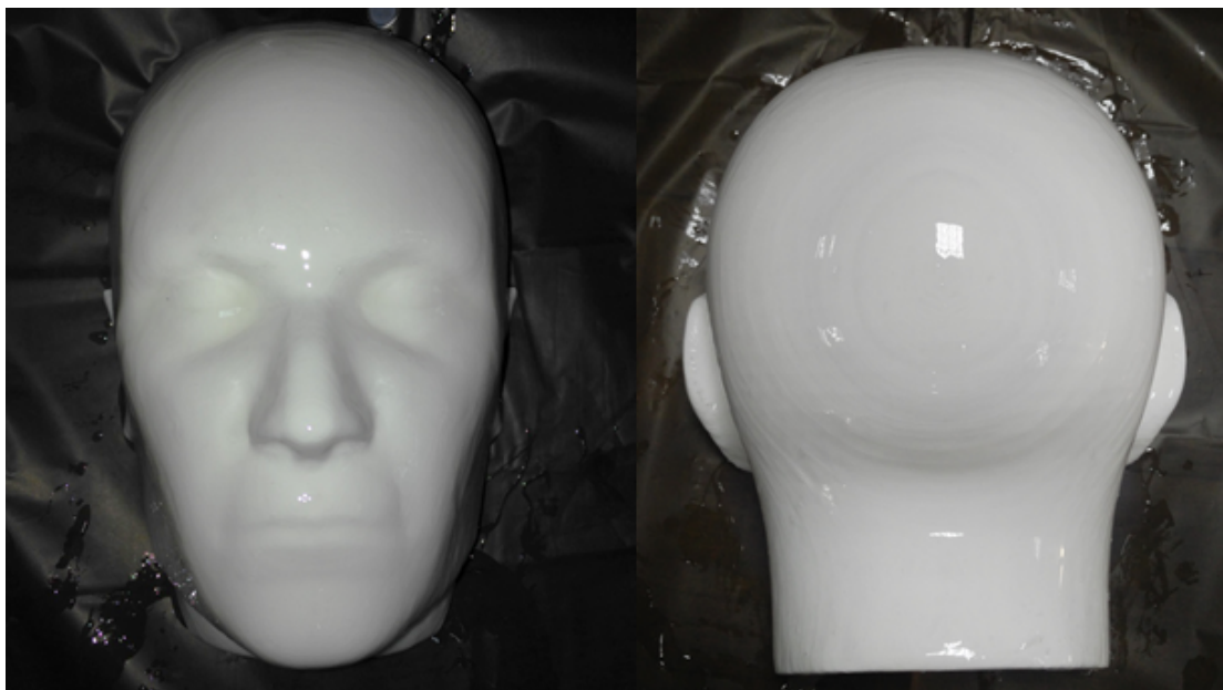
Figure B.2: The 3D printed head parts after applying the soft material.
