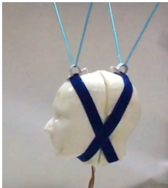
Figure B.6: The dummy head after assembling it with the Velcro straps.
