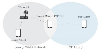
Figure 2.5 Wi-Fi direct architecture.
