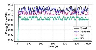
Figure 4.8 Energy efficiency (single UAV).
