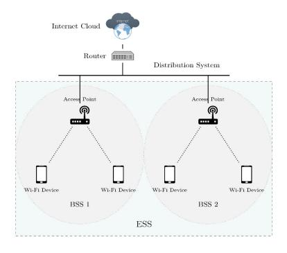
Figure 2.1 WLAN architecture.
