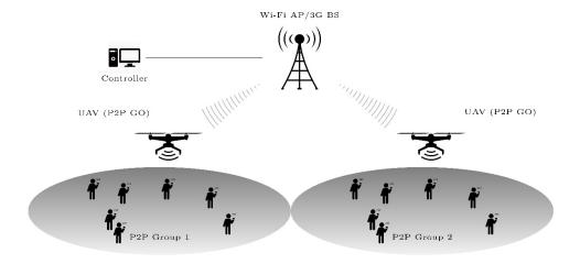
Figure 4.1 UAV-aided Wi-Fi direct network architecture.
