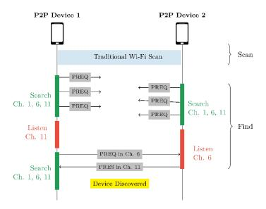
Figure 2.6 Device discovery procedure in Wi-Fi direct.
