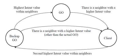
Figure 3.2 Device state diagram for BGO selection.
