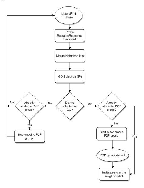
Figure 3.1 Device state diagram.
