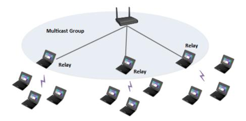
Figure 2.4 Multicasting with cooperative relaying.
