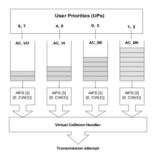
Figure 2.2 EDCA channel access scheme.
