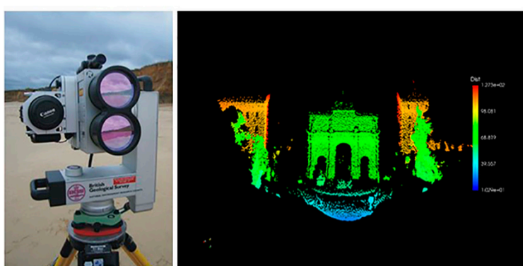
Figure 5. LiDAR scanning equipment and scanning result (Courtesy of Blickfeld, 2018).
