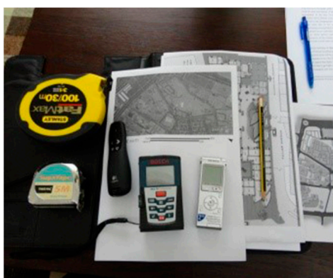
Figure 4. Conventional tools used in terrestrial (manual) survey (authors, 2012).
