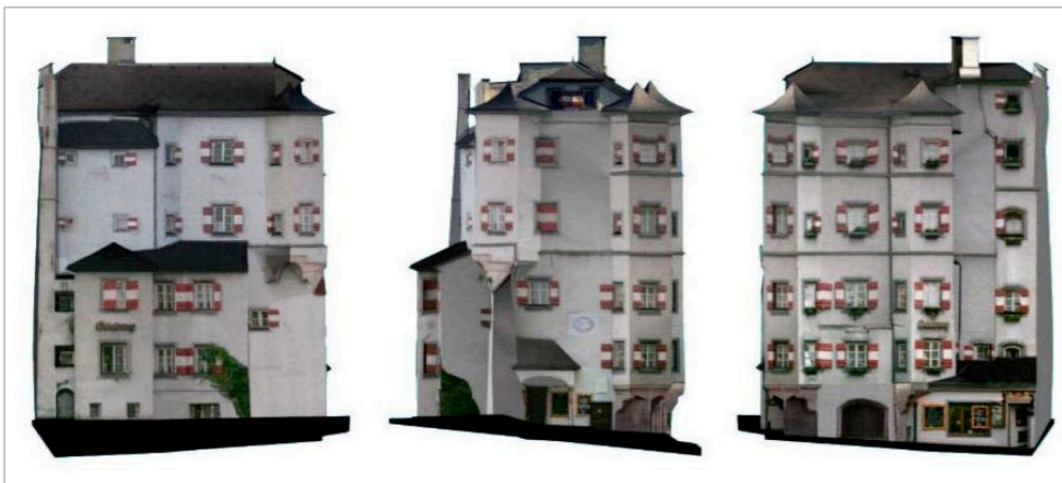
Figure 3. Photogrammetry—3D model of historical building (source: Hanke & Grussenmeyer Corfu, 2002).
