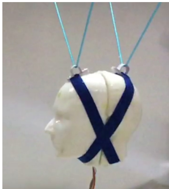
Fig. 6. The dummy head after assembling it with the Velcro straps.
