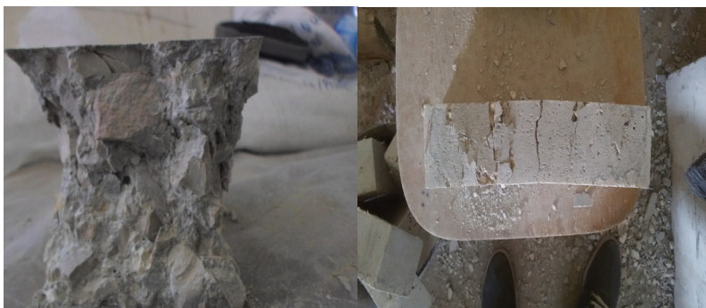
After compressive test
