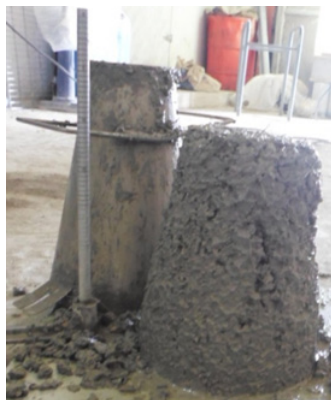
Figure 4: Slump test realized on recycled PP fibers concrete
