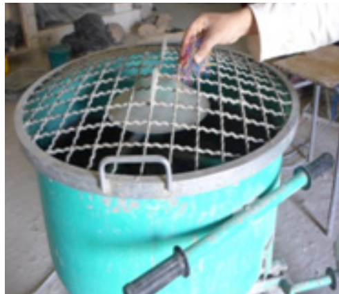
Figure 2: Adding of PP fibers
