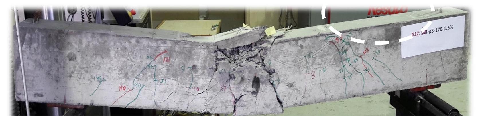
Beam with 1.5% of fibers (Compression flexural failure without concrete spallation)
