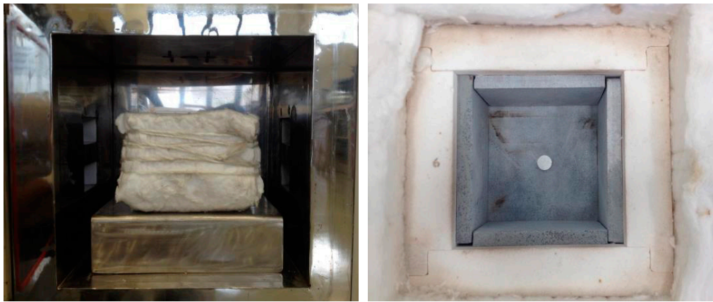
Figure 5. (a) Susceptor cavity inside the furnace; (b) Susceptor showing SiC lining [27].
