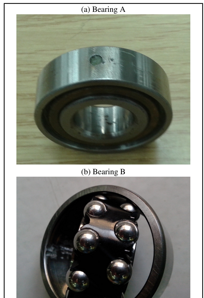
Figure 5. Notches in the outer races of bearings A and B.
