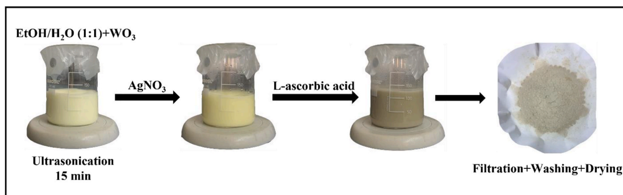
Scheme 1. The schematic diagram for the preparation of 1% Ag/ \text{WO}_3 catalyst.
