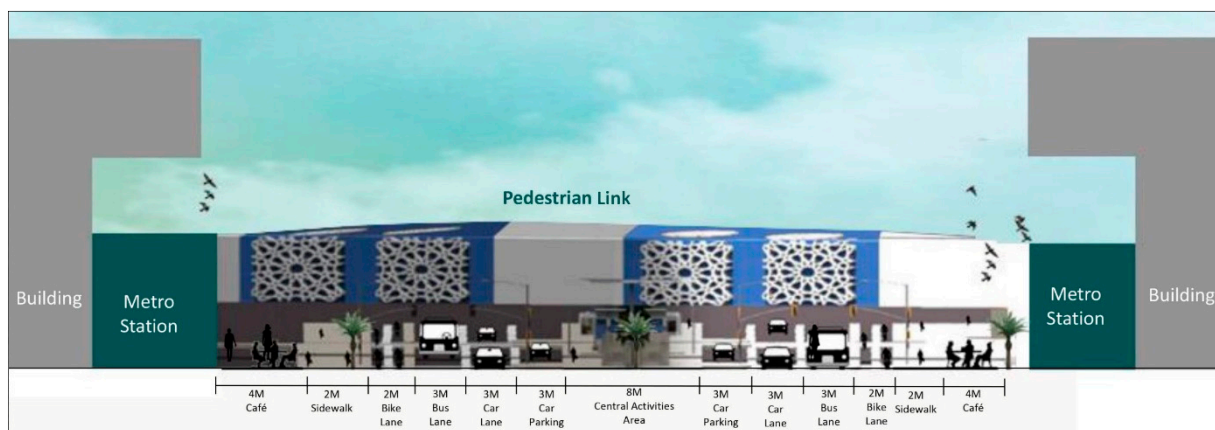
Figure 25. New proposed street cross section, aiming to achieve a multimodal transportation system that is integrated with outdoor spaces (Source: the Authors).
