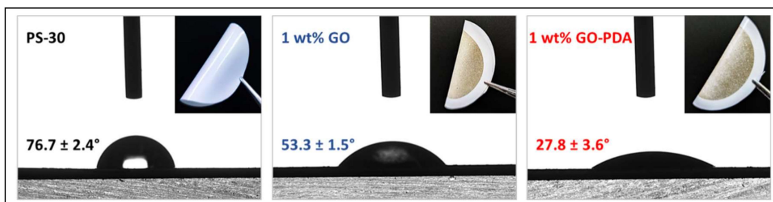
Figure 13. Contact angle of PS-30, PS/GO, and PS/GO-PDA membranes.
