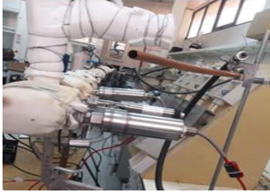
Figure 32. Side view of the mounting of the pressure transducer on the tube
